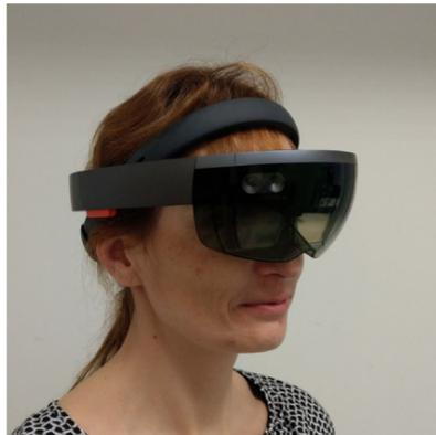
Head mounted device (HMD) HoloLens 1®
